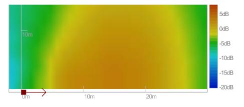
(b) SA250S horizontal directivity: sound level for the voice octaves (500Hz,1kHz,2kHz) on the listening plane.
