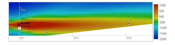
(a) SA180S vertical directivity: sound level for the voice octaves (500Hz,1kHz,2kHz) in the vertical median plane.
