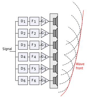
(a) In a geometric array, loudspeakers are aligned along the shape of the wave front to be generated, usually a J shape.
