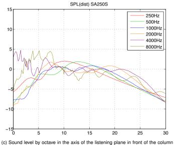
(c) Sound level by octave in the axis of the listening plane in front of the colum with respect to the distance from the column.
