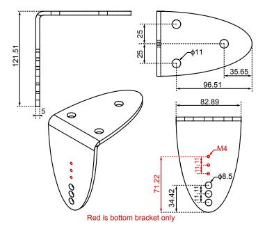
Figure 18: Fixing brackets for wall mounting of StepArray columns.
