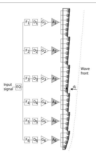
Figure 4: The DGRC principle used by StepArray columns. The wave front is controlled both by the positioning and orientation of the loudspeakers, and by filters  $F_i$ , delays  $D_i$ , and gain  $G_i$  of each channel.
