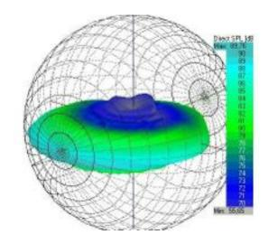
(b) Balloon plot of SPL radiated in octave 1 kHz by column SA250S. Simulation with EASE®.
