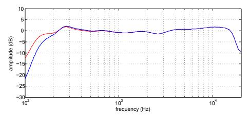
Figure 19: Frequency response (column SA250P). Average of the mesurements at 7, 10, 15, 20, 25, and 30m. In red: with bass high-pass on position «100Hz», in blue: with bass high-pass on position «200Hz».
