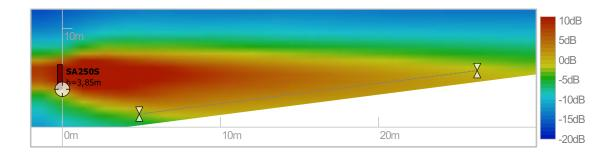
(a) SA250S vertical directivity: sound level for the voice octaves (500Hz,1kHz,2kHz) in the vertical median plane.
