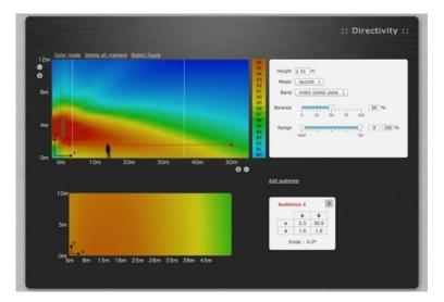
Figure 11: StepArray directivity control with the NUT software
