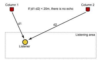
Figure 10: Interferences between columns
