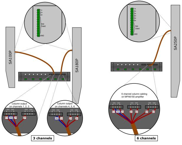
Figure 16: MPA6150 to column wiring
