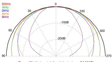
Figure 20: Horizontal directivity (column SA250P)
