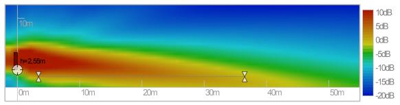
(a) SA250P vertical directivity: sound level for the voice octaves (500Hz,1kHz,2kHz) in the vertical median plane.
