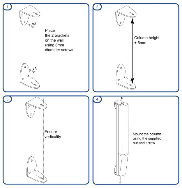
Figure 13: Column mounting on a wall
