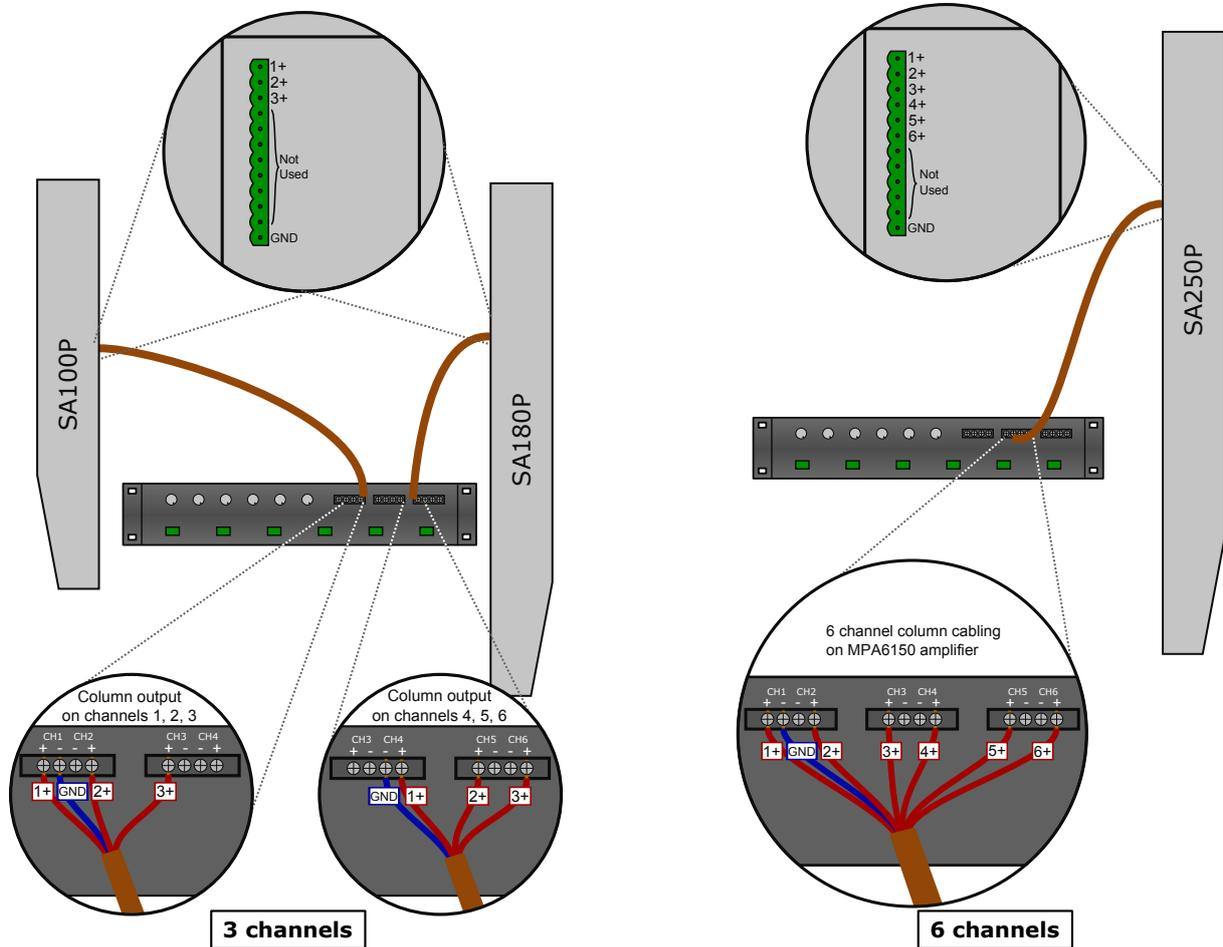
Figure 16: MPA6150 to column wiring
