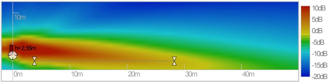
(a) SA180P vertical directivity: sound level for the voice octaves (500Hz,1kHz,2kHz) in the vertical median plane.
