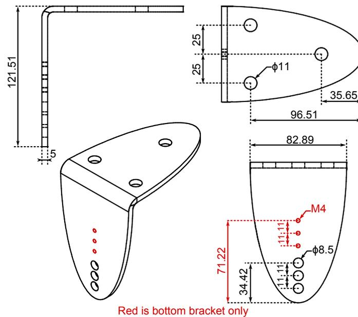
Figure 18: Fixing brackets for wall mounting of StepArray columns.
