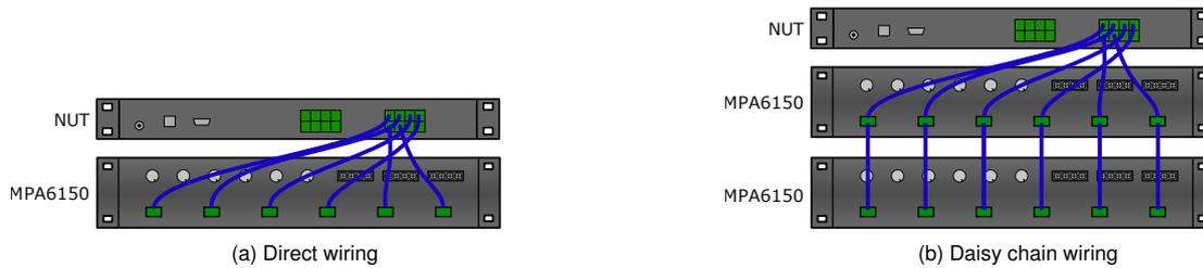
Figure 14: NUT to MPA6150 wiring
