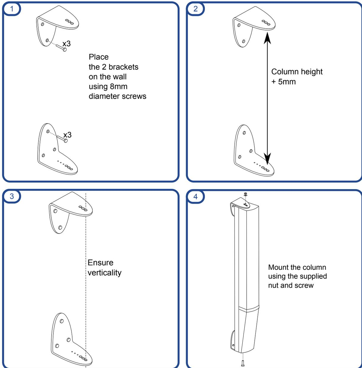
Figure 13: Column mounting on a wall
