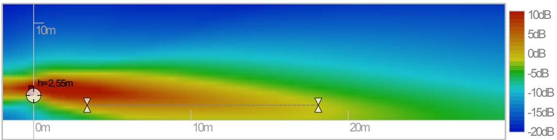
(a) SA100P vertical directivity: sound level for the voice octaves (500Hz,1kHz,2kHz) in the vertical median plane.
