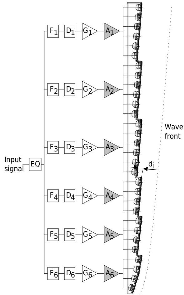
Figure 4: The DGRC principle used by StepArray columns. The wave front is controlled both by the positioning and orientation of the loudspeakers, and by filters  $F_i$ , delays  $D_i$ , and gain  $G_i$  of each channel.
