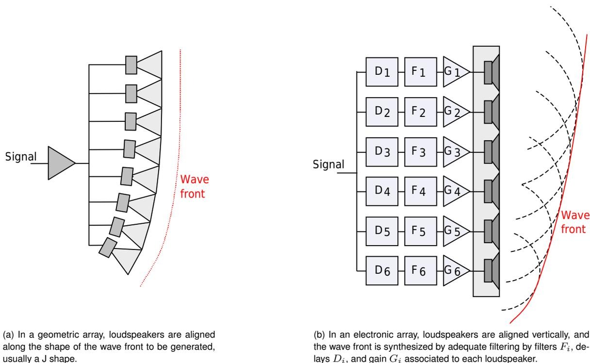
Figure 3: Electronic and geometric arrays
