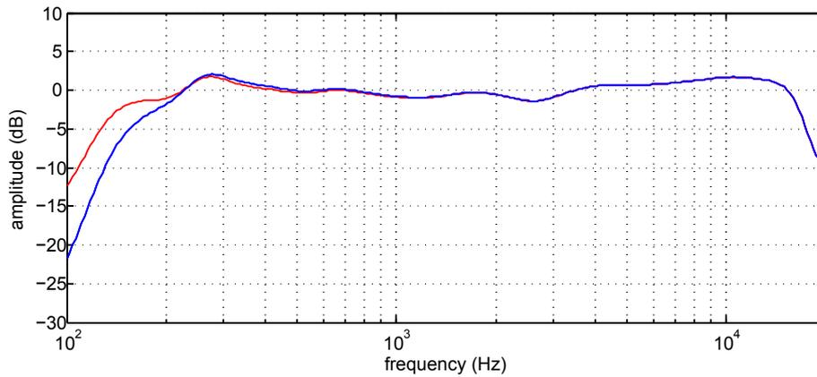
Figure 19: Frequency response (column SA250P). Average of the measurements at 7, 10, 15, 20, 25, and 30m. In red: with bass high-pass on position «100Hz», in blue: with bass high-pass on position «200Hz».
