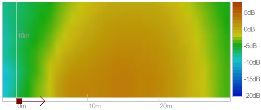
(b) SA250S horizontal directivity: sound level for the voice octaves (500Hz,1kHz,2kHz) on the listening plane.
