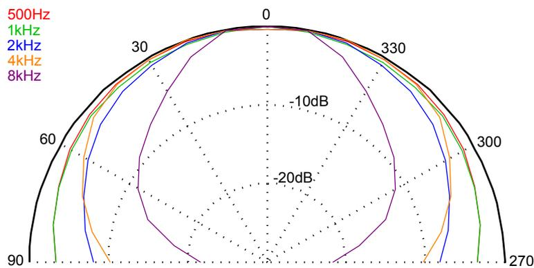
Figure 20: Horizontal directivity (column SA250P)
