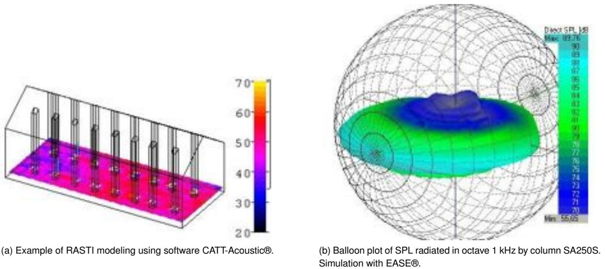
Figure 12: Examples of a CAD modeling results.
