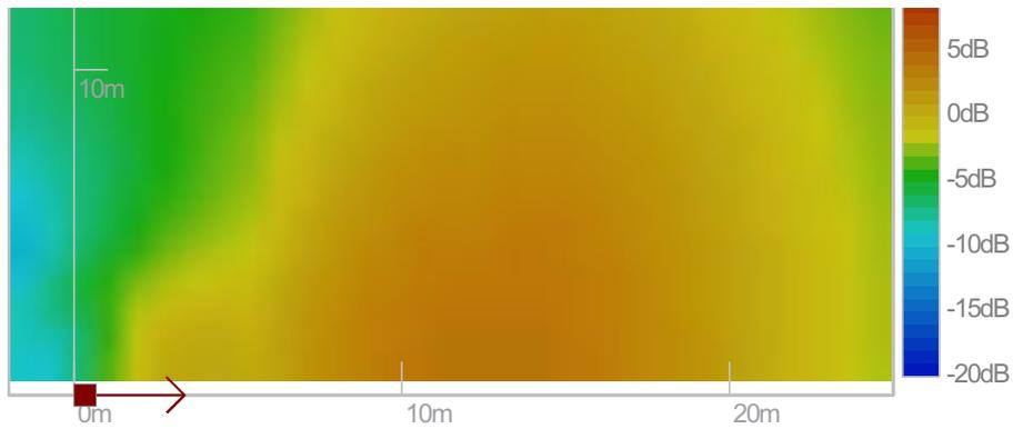
(b) SA180S horizontal directivity: sound level for the voice octaves (500Hz,1kHz,2kHz) on the listening plane.
