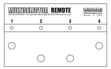
The optional MultiSelector MLTSELPRO4XR Remote "stomp box" style footswitch contains four switches that remotely control the switching functions of the rack mount unit using a regular 3pin XLR microphone cable. A unique, proprietary communication protocol ensures reliable switching with mic cables up to 100 feet long.
