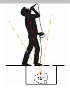
$15^\circ$  angle for under stage. This solution is often used on TV stages to hide the monitor speakers. From approx. 0.5m to 1.5m.
