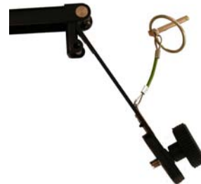
(2) Remove locking pin on the pivoting arm
