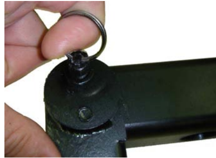
(2) Release pivoting arm locking pin
