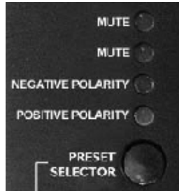
Figure 8: SB15P preset selector switch closeup
