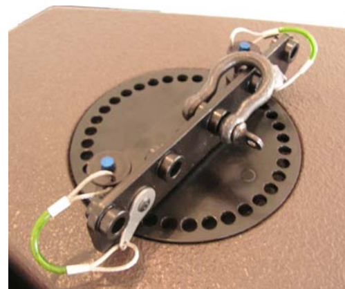
(4) Two locking pins are used to secure the XTLIFTBAR. Shackle locations (front to back) provide +18, +11, +3, -5, -13 degree tilt angles, respectively
