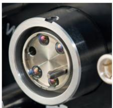
Waterproof up to 10 m (33 ft) for 12 hours PG cable relief Highly resistant black finishing Roller studs for easier coupling High resistance to shock and vibrations Expanded beam fiber optic contacts Easy and error-free mating Audible snap in quick bayonet lock Excellent resistance against unlocking
