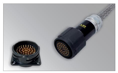
LKA 48/6 was designed to connect speaker clusters to their amplifiers utilizing the least possible number of cables, up to 24 speaker channels using a cable with a 4mm2 section, Eurocable 36N40AD2 or 48N40AD2. Additionally, there are 2x AES/EBU channels for laser pointing and inclinometer control, and the LKA 48/6 features a mesh cable gland as standard for maximum durability.
