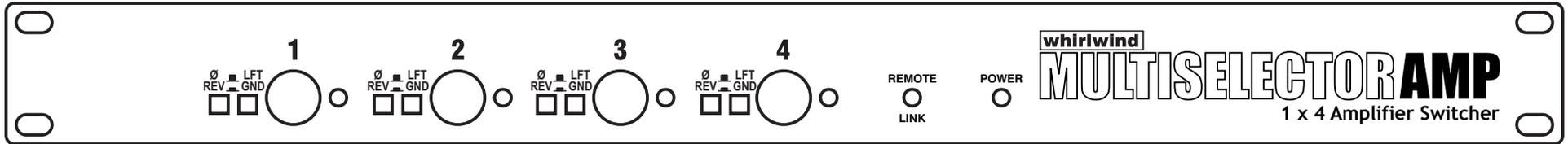
Four momentary switches on the front panel turn the channels on and off, with each active output identified by a blue LED. All four outputs of the MultiSelector AMP can be on at the same time. A separate green LED indicates connection of the optional foot controller, the MLTSELAMPR Remote.
