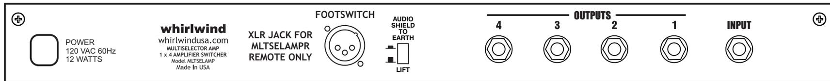
The rear panel contains the 1/4" input jack, the four unbalanced 1/4" output jacks, and a male XLR connector for connecting the optional remote footswitch. The unit is AC powered for ultimate performance and no "wall wart". The standard version MLTSELAMP is set for 120 Volt operation. The MLTSELAMPX version is set for 230 Volt 50/60Hz operation.
