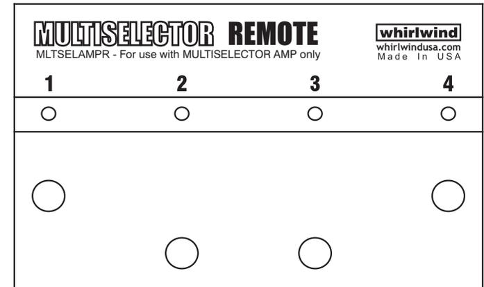
The MultiSelector MLTSELAMPR Remote "stomp box" style footswitch contains four switches that remotely control the switching functions of the rack mount unit using a regular 3 pin XLR microphone cable. A unique, proprietary control protocol ensures reliable switching with mic cables up to 100 feet long.
