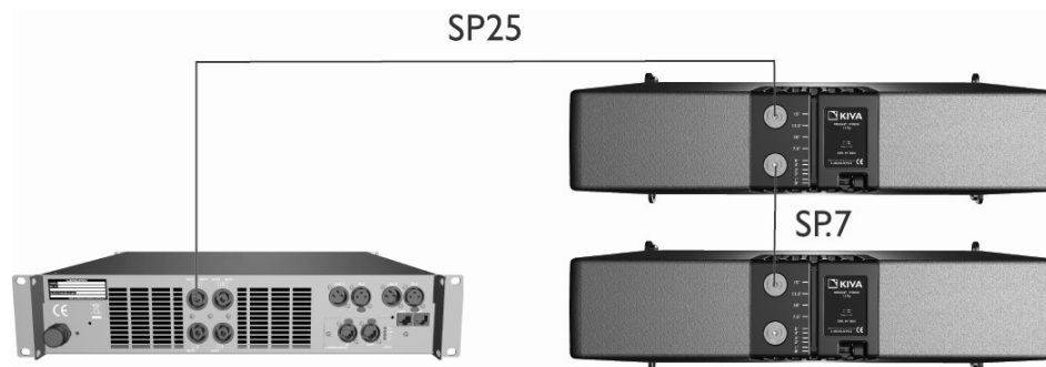
Figure 3: Connecting two KIVA in parallel to an LA4 amplified controller
