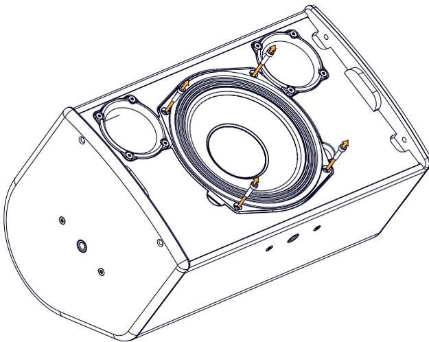
2. Remove the speaker assembly carefully and disconnect the speaker cables.
