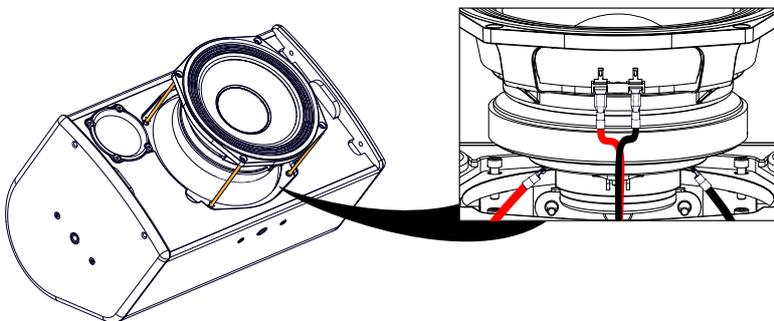
3. Secure the speaker with the S342 screws.
