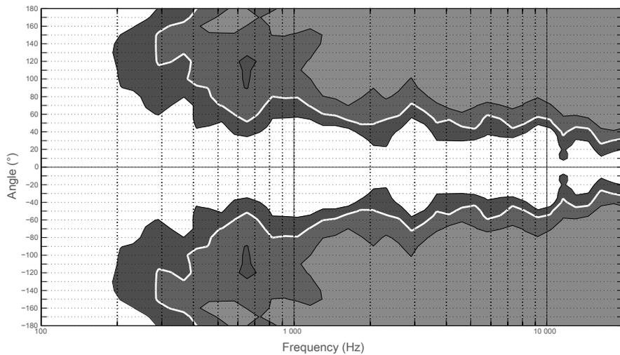
Dispersion angle diagram of a single X8 using lines of equal sound pressure at -3 dB, -6 dB, -12 dB.
