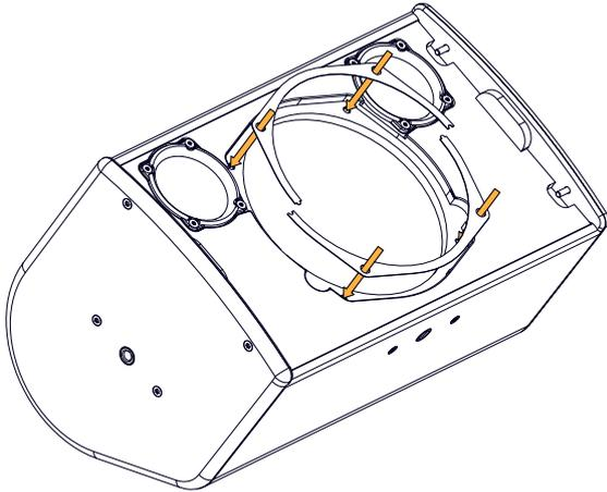
2. Connect the speaker cables and position the speaker.
