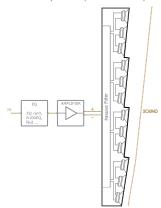
Ray-On is based on the DGRC principle: the internal loudspeaker inclination associated with the calculated height of installation allows to cover the audience area.
