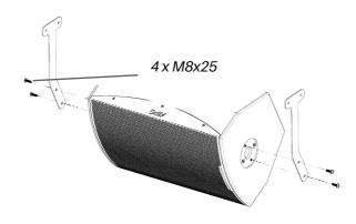
2. Assemble by approaching the iX12 under the iS115 then fix the junction pieces to the iS115 using the M8x25 screws.
