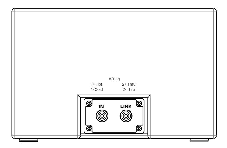
The rear panel of the iS Series subwoofers are equipped with two NL4 connectors. The four pins of the two connectors are connected in parallel. The speakers occupy points 1 + / 1-.
