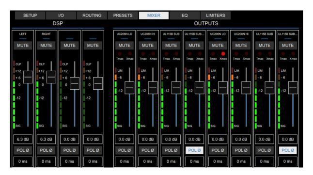
The LIM LED displays the activation of the Vx limiter.
