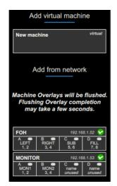
This button opens a menu allowing you to add machines available on the network, as well as virtual machines to prepare an offline configuration by simply clicking on the machines panels.
